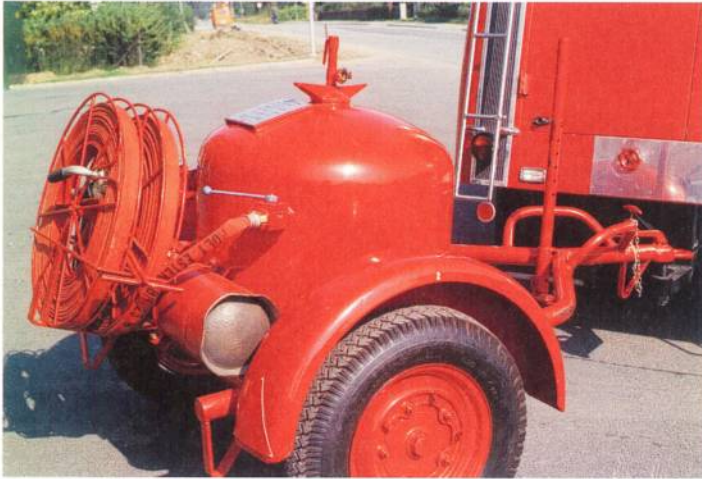
4.2 Powder units are probably the most powerful extinguishing resource the fire service has available.
