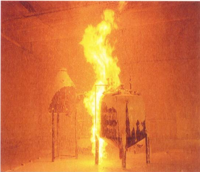
3.23 Fire suppressed by foam sprinkler in an industrial process. Sometimes manual extinguishing is also required at the fuel outlet.
