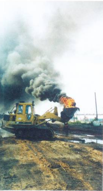
1.3 The burning material can be moved away to make extinguishing the fire easier.
