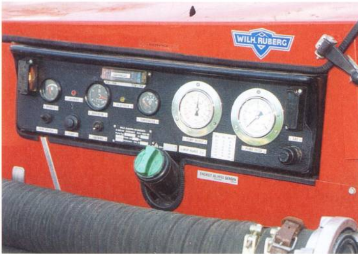
2.18 Control panel for a trailer pump including a vacuum gauge and manometer. Note the sign with the conversion factors for different units of pressure.
