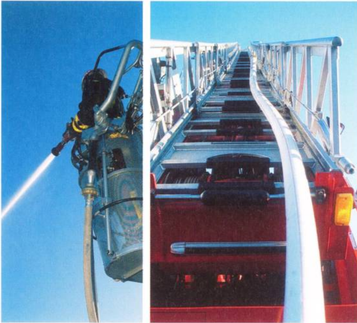
2.47 When laying out a hose on a ladder, the hose is always positioned to one side. The attack hose is fastened in position and can hang freely.
