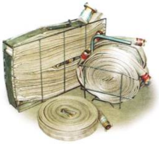
2.42 Hoses can either be rolled or folded for storage. Rolled hoses are either single-rolled or double-rolled. Folded hoses need some sort of storage equipment.
