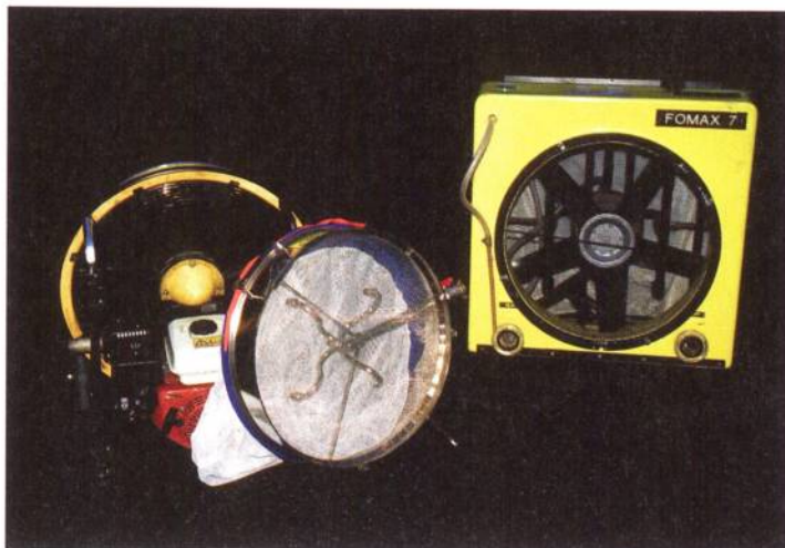
3.30 Fan for positive pressure ventilation with a high-expansion foam attachment and high-expansion foam unit respectively.
