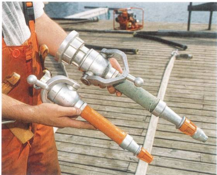
2.57 A small jet/spray branchpipe with a claw coupling and a large one with a normal coupling. The branchpipe is closed if the handle is pushed forward. If the handle is vertical it produces a water spray and with the handle facing backwards a solid jet.
