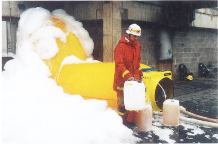
3.32 Using a high-expansion foam unit with a hose and door adapter.
