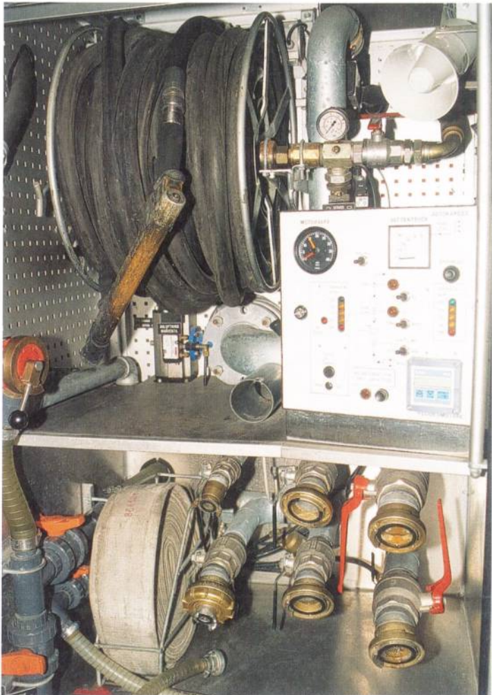
2.19 A fire engine equipped with a pump with a high-pressure hose reel and low-pressure outlet, together with equipment for mixing foam. Note that the pump has a flow meter. With a feeder pump, it can also take water from a static water supply.
