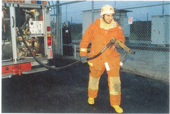
2.36 A semi-rigid hose on a reel has advantages when speed and flexibility are crucial.
