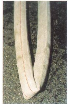
2.49 If a kink forms in a hose, this will cause significant wear.
