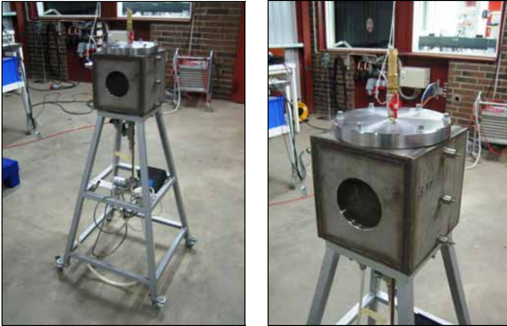
Figure 8 Explosion chamber ("bomb"), volume of 8 \text{ dm}^3 , which was used for the explosion tests.
