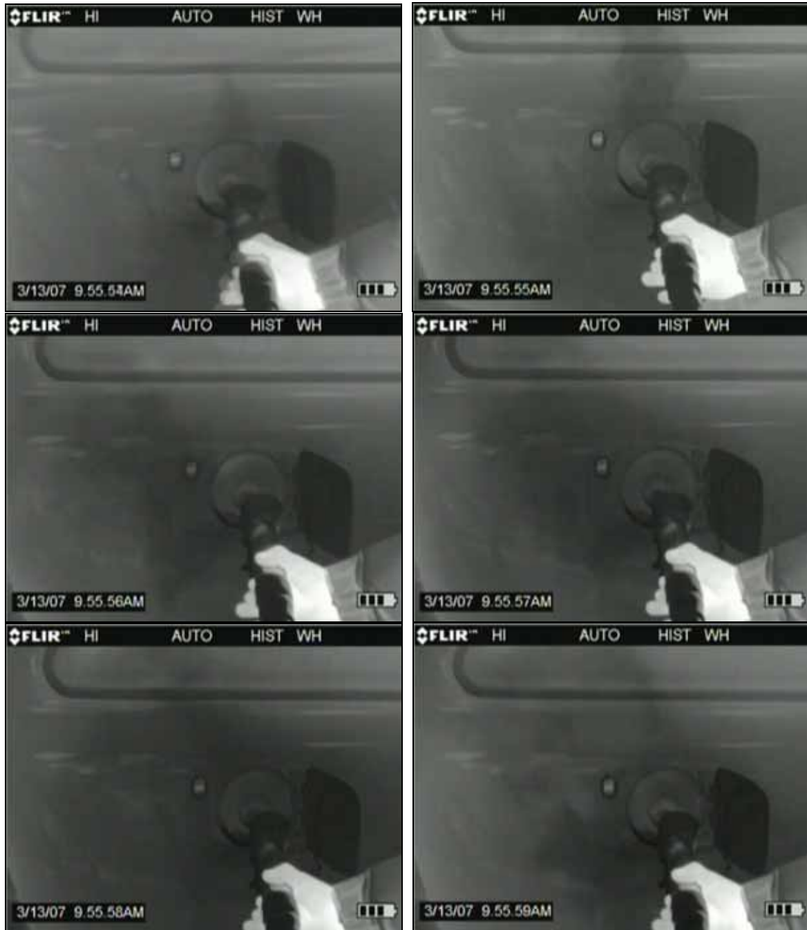
Figure 36 Examples of picture sequences from the GasFindIR camera during refuelling without the vapour recovery system activated. Emission of the fuel vapours can be seen as grey-black “smoke” on the pictures (selected photos from a 6 second video sequence).
