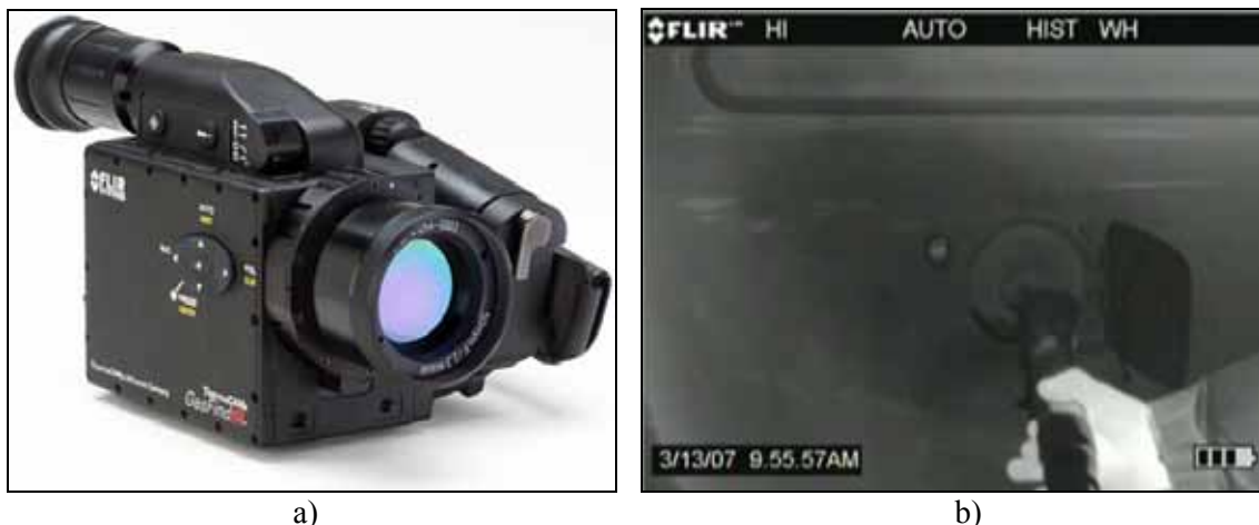
Figure 34 a) IR camera GasFindIR from FLIR Systems AB which was used to obtain a coarse picture of the gas emissions around the refuelling opening during tanking. b) An example of the type of picture that the camera shows where the dark grey area to the left of the refuelling opening indicates the presence of fuel vapour.
