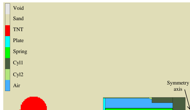
Fig. 4 The material location of the 2D axis symmetry model. The colours void, blue, green, cyan, red, purple, and yellow corresponds to the materials, sand, TNT, plate, spring, cyl1, cyl2 and air.
