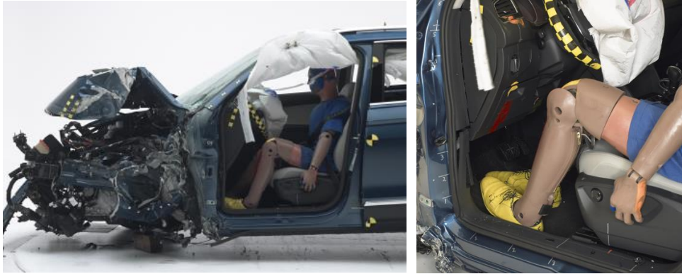
Figur 44. Small-overlap prov med 2018 Volkswagen Tiguan (MQB plattform)
