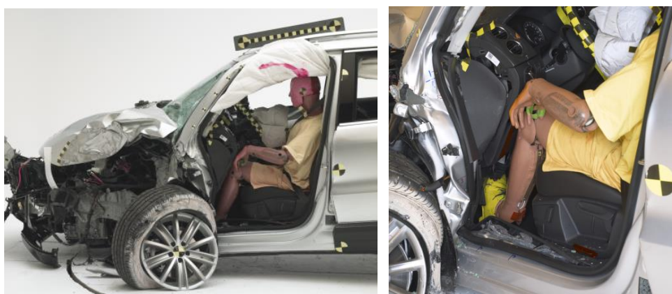
Figur 43. Small-overlap prov med 2013 Volkswagen Tiguan (PQ46 plattform)
