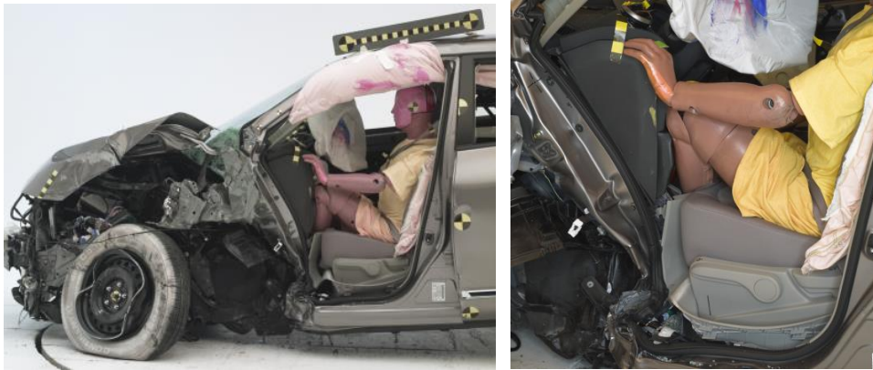
Figur 40. Small-overlap prov med 2012 Nissan Qashqai (C plattform)
