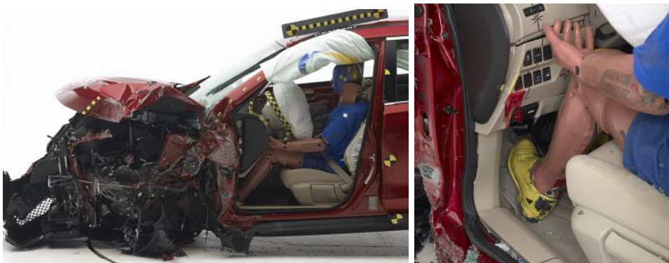
Figur 41. Small-overlap prov med 2014 Nissan Qashqai (CMF plattform)
